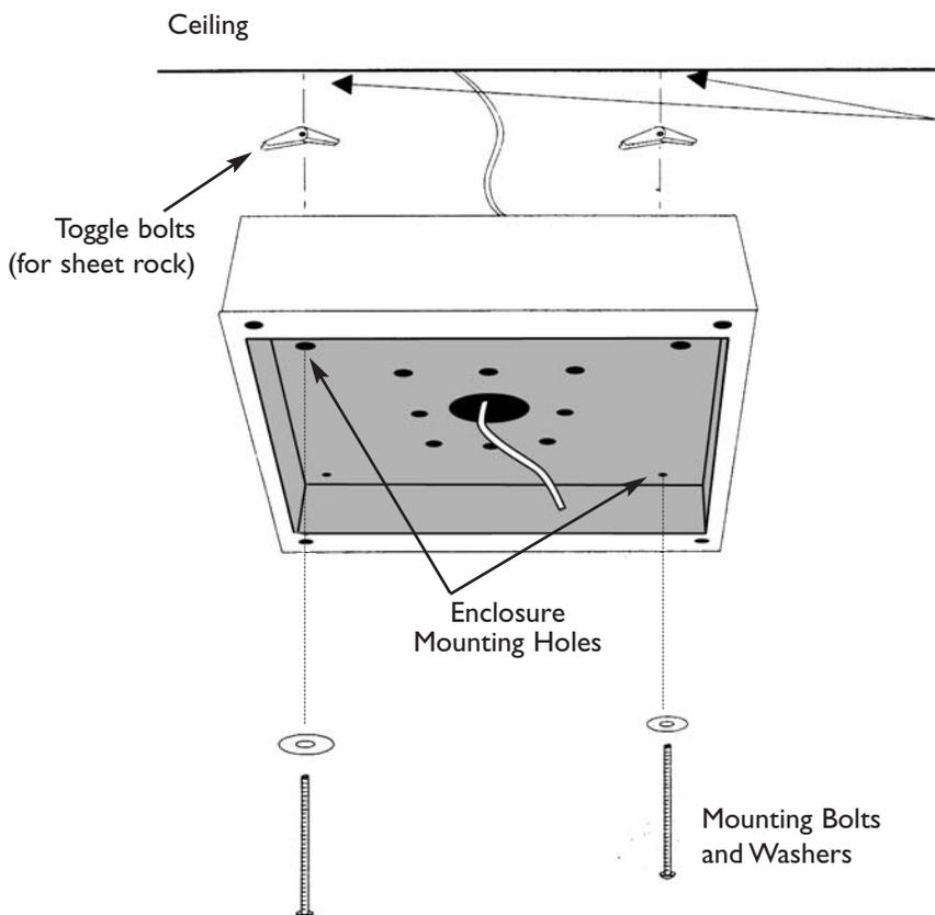
Use two of the enclosure mounting holes as a template (diagonally opposed), and mark screw hole locations. If toggle bolts will be used, use a drill to cut two, 1/2" diameter holes in the ceiling.
