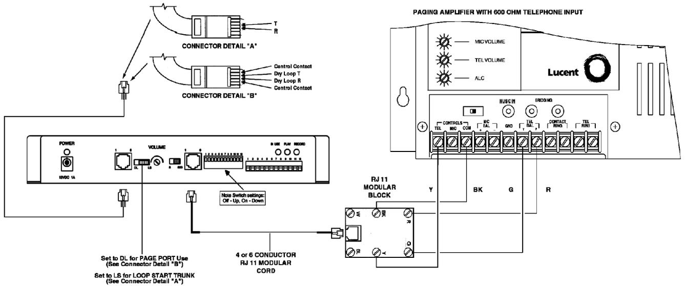
Figure 2-2. Digital Feedback Eliminator Interface with Telephone Paging Amplifier
