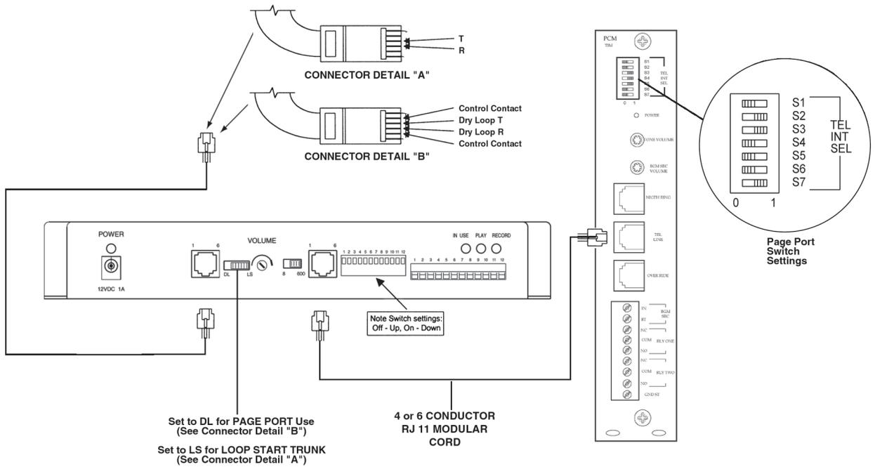
Figure 2-1. Digital Feedback Eliminator Interface with LUPCM Zone Paging System
