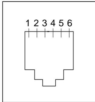
Figure 2-3. RJ12 Connector
