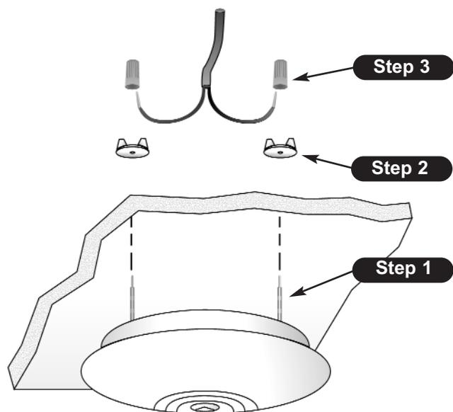
**STEP 1** - Set speaker tap to correct setting using the *Tap Settings* chart. Position the speaker on the ceiling tile and slowly push the speaker, forcing the studs through the ceiling tile.
